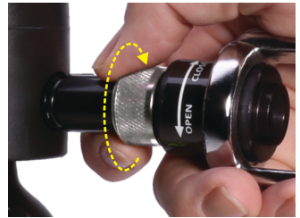
(4) Turn bleed ring to closed position.
