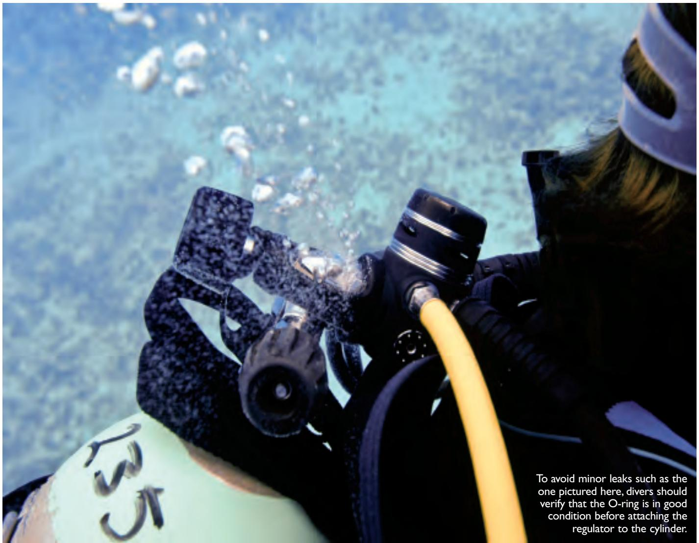
To avoid minor leaks such as the one pictured here, divers should verify that the O-ring is in good condition before attaching the regulator to the cylinder.
